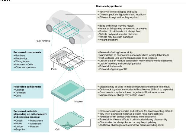
$\textbf{Fig. 4} | \textbf{Diagram showing challenges of disassembly at different levels of scale.} \\ \textbf{Electric-vehicle battery packs are complex in design, containing wiring looms, bus bars, electronics, modules, cells and other components.} \\ \textbf{There are } \\ \textbf{There are } \\ \textbf{There } \\ \textbf{T$
