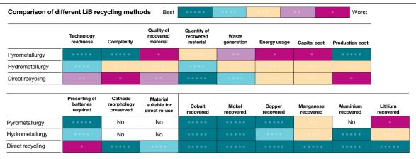
Fig. 6 | Comparison of different LiB recycling methods.
